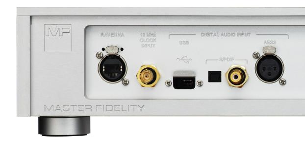
Connection Wanted: In addition to the usual interfaces, the NADAC D includes two less common ones—visible on the left in the picture. Ravenna, a nod to the unit's studio pedigree, is joined by a BNC socket for the external master clock, the NADAC C.
