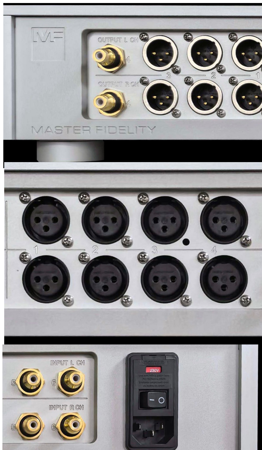
Everything in its place: six line-level inputs, four pairs of outputs, and the power section.
